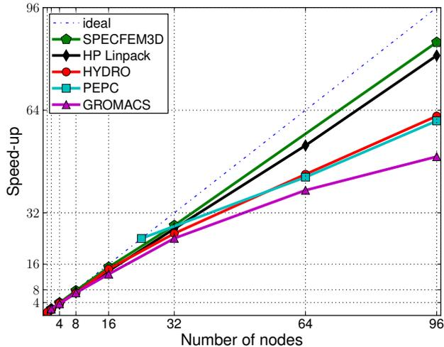
**Figure 6: Scalability of HPC applications on Tibidabo.**
