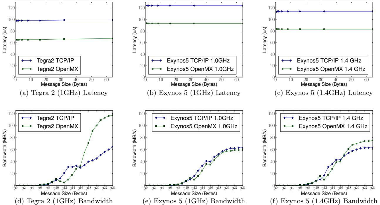
Figure 7: Interconnect measurements
