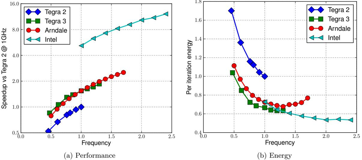
Figure 4: Multi-core performance and energy efficiency results of micro-benchmarks with frequency sweep. Baseline is the Tegra 2 platform running at 1GHz.
