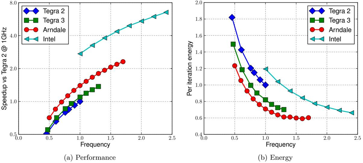
Figure 3: Single-core performance and energy efficiency results of micro-benchmarks with frequency sweep. Baseline is the Tegra 2 platform running at 1GHz.
